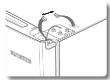
2. Disconnect electric wire on the top of the refrigerator.
